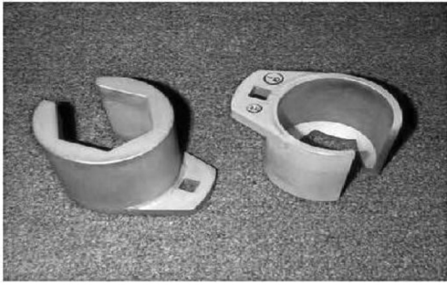
212/412 Main Hydraulic Servo Alignment Tools HTI007
