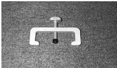
212/412 Tail Rotor Hub Trunnion Centering Tool HTI011
