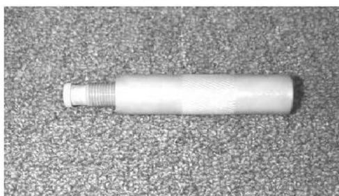
204/205/212/412 Swashplate Gimbal Ring Bolt Removal Tool HTI012
